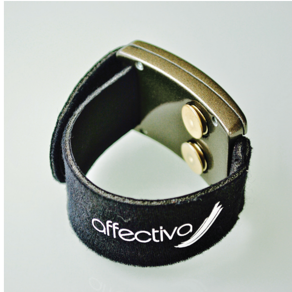
Fig. 1. Off-the-shelf Affectiva Inc. Q Sensor, with electrodes to measure EDA at the back
